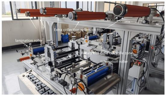
**5,Collection rollers** ,the collection rollers will collect the kiss cut velcro or different slitted width velcro into rolls
